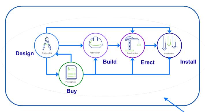
**Enterprise 2.0**. McDermott utilizes 3D model based end to end (E2E) integrated design-buy-build enterprise software to design, procure, fabricate and construct onshore and offshore facilities.
